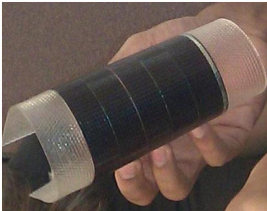
*This is the high-efficiency Alta Devices solar cell.*
