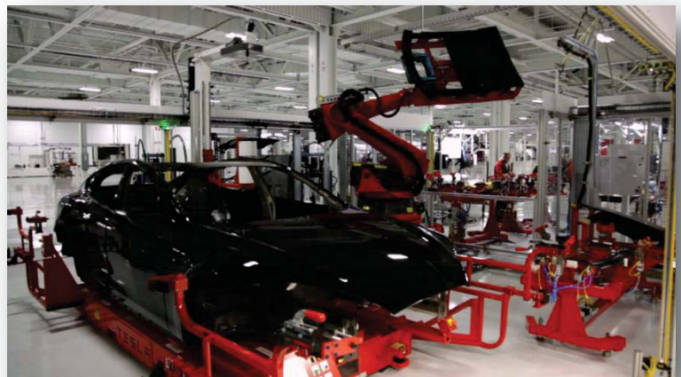
Robotic Installation of Panoramic Roof
